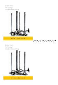
Engine valves are used in most piston engines to open and close the intake and exhaust ports in the cylinder heads. The valve is usually a flat disk of metal with a long rod known as the valve stem out one end. Engine valves usually made up of silicon alloy steel. Nowdays stellite alloys are used much to increase the wear resistance and for operations high temperatures. Valves are processed with nitidization or chrome or titanium platting to harden the surface and stem.
